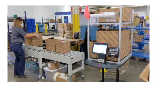
Within the aisle, 6 River Systems autonomous mobile robot Chuck, supports packing custom quantities of SKUs with an integrated mobile printer and accessory bag dispenser. When orders are fully picked and hit the conveyor at unloading, Legend Valve's ERP, JD Edwards, is updated with the status.
