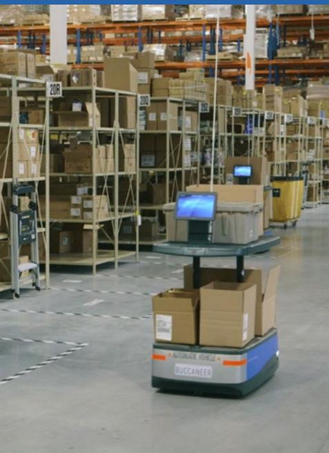
In 2019 and 2020, the company introduced more than 100, 6 River Systems' autonomous mobile robots, Chucks, across their five strategically located distribution centers, replacing their old in-line conveyor systems and enabling the distributor to rethink the workflow of their warehouses.
